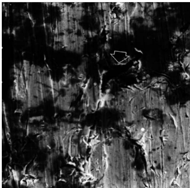
Figure 7. AISI 304 (1,000 \times ): crevice corrosion due to the formation of occluded area.
