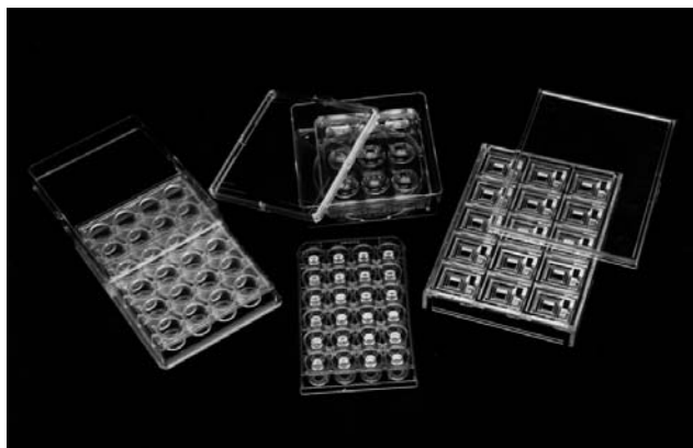
Figure 14. Four examples of trays, plates, or combinations used for crystallization by vapor diffusion. All are commercially available and can be used for either the hanging-drop or the sitting-drop approach.
