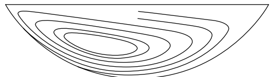
Figure 10. Pathlines of six particles with settling velocity of V_s = 0.05 U placed in the flow.
