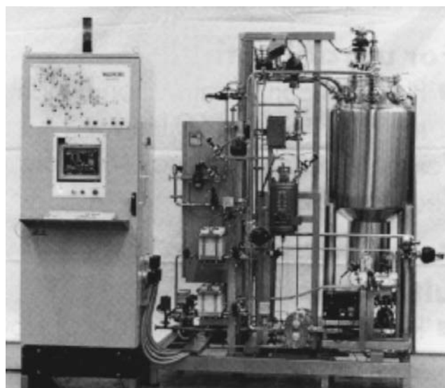
Figure 18. A fully automatic system with several membrane cassettes for protein concentration. Source: Photo courtesy Millipore S.A., Molsheim, France.
