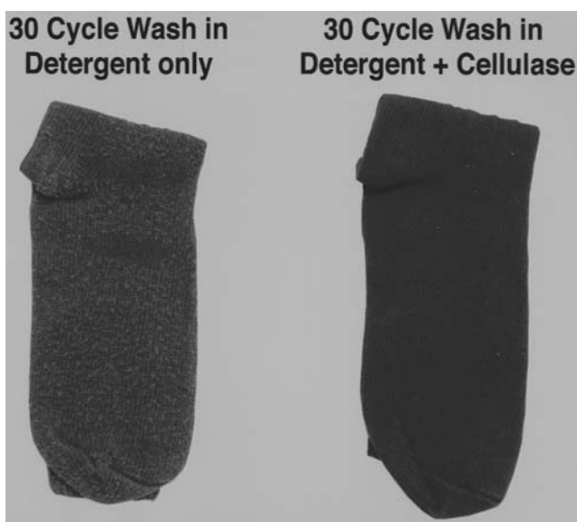
Figure 8. Effect of Carezyme® after 30 wash cycles. (a) 30-cycle wash in detergent only; (b) 30-cycle wash in detergent plus cellulase.
